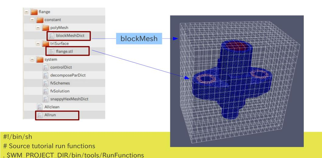
runApplication blockMesh runApplication surfaceFeatureExtract -includedAngle 150 -writeObj constant/triSurface/flange.stl flange runApplication snappyHexMesh -overwrite
